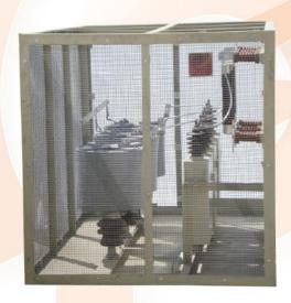
Medium voltage capacitor bank for industrial application can be offered with Series / Neutral End Reactors, Neutral Current Transformers / Residual Voltage Transformers and HRC Fuses, enclosed in wire mesh or sheet steel enclosure for indoor / outdoor installations as per requirements.
